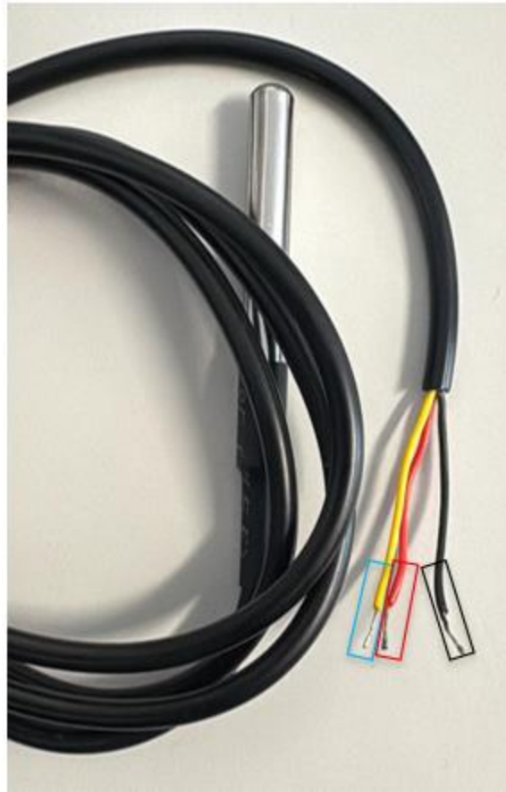
Figure 5: I/O part with negative, positive and signal pins indicated
